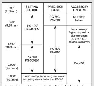
Inquire about special gages and setting fixtures for diameters to 4.300" (109 mm)
