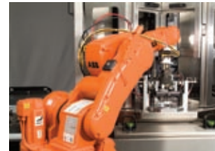
MULTI-AXIS SERVO ROBOT SHOWN INTEGRATED INTO A SUNNEN MODULAR HONING SYSTEM.
