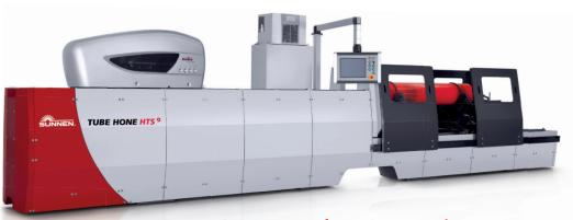
**Sunnen Tube Hone series** is the result of more than 30 years experience in tube hone design and manufacturing. Most of the systems are custombuilt and have enough power and sensibility to work from diameter 4 mm up to 1'000 mm.
