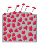
Figure 2: Each grain breaks out of its bond precisely when the grain point is blunt.
