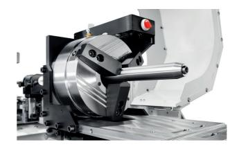
The **pneumatic three-jaw chuck** simplifies part changes and saves valuable time. A manual three-jaw chuck is also available for less productive applications.
