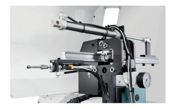
The **in-process plug gauge** is reliable and independent of stone wear in holding tightest tolerances. The long-life carbide probe controls on reverse stroke with an accuracy of up to 0.002 mm.
