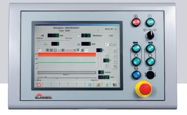
**Intuitive touch control** with clear, self-explanatory screen. It is the ideal system for optimized process control and fits in all production industries. No programming skills required. A new set-up can be made within 2 minutes, step-by-step. The system recommends the required tool, sets the spindle speed and all necessary cycle parameters. All parameters can be stored.
